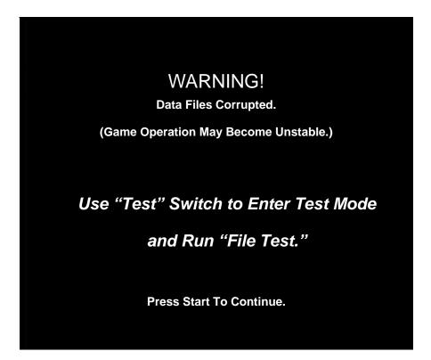
**CORRUPT FILE SCREEN.** If you see the above screen, your VIDEO GAME MACHINE computer has corrupt files. To determine which files are corrupt, you can run the File Test. (See *Chapter 3, Audits, Adjustments & Diagnostics.*) The File Test can't repair corrupt files, though. The only solution is to perform a hard-drive recovery.
