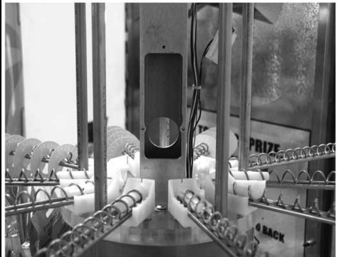
motor removed from center post
