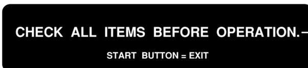
The message “CHECK ALL ITEMS BEFORE OPERATION.” appears at the bottom of the “ALL FACTORY SETTINGS” screen, when the existing settings have been returned to their factory ones, to prompt you to make all the necessary settings. Press the 1P start button to return to the main menu screen.
