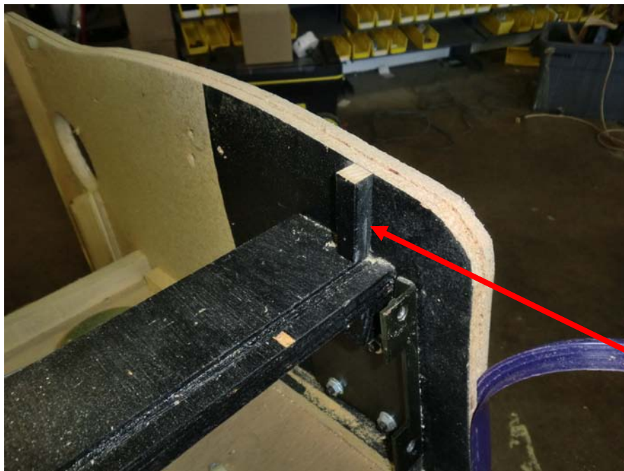
Figure 20 - New Groove Should Match Original
