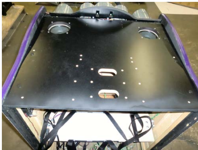
Figure 58 – Install Top Panel
