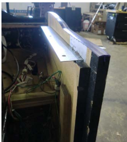
Figure 56 - Install Long L-Brackets (World & Exotica shown)
