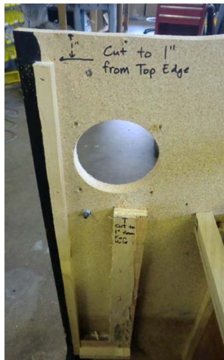
Figure 22 - After Cleats are Removed & Plywood is Cut
