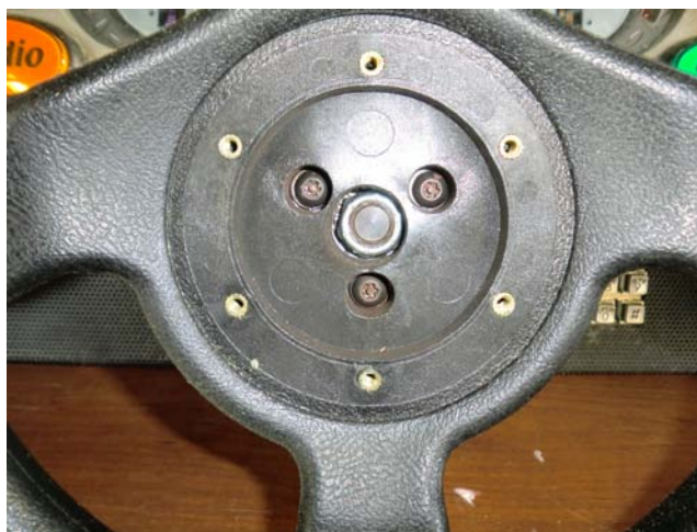
Figure 37 - Remove 3 Screws and Steering Wheel Hoop
