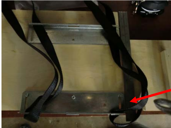
Figure 51 - PC Strapping Parts (plus Foam Pad)
