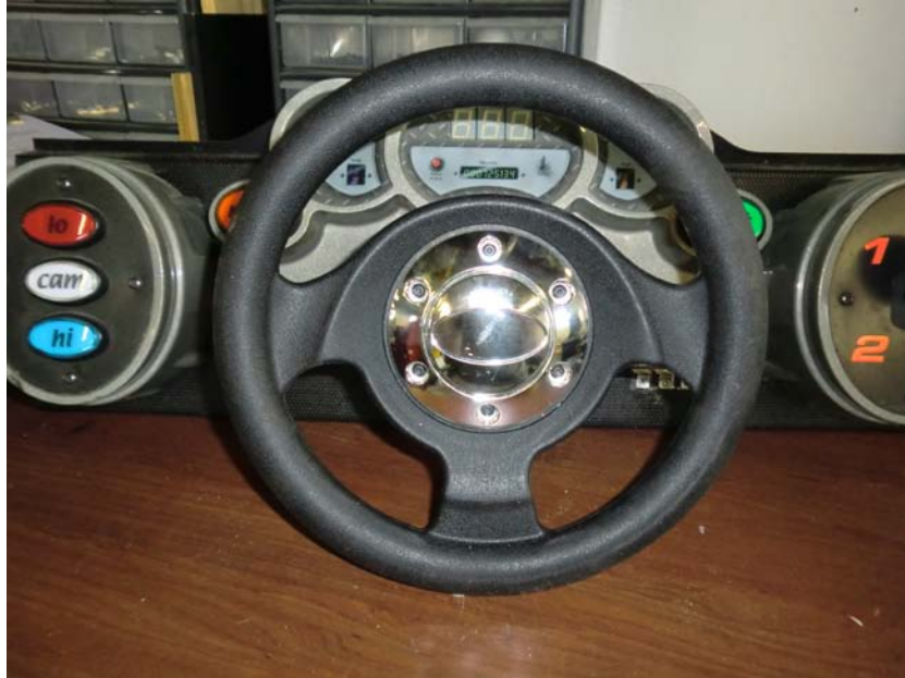
Figure 43 - DO NOT OVERTIGHTEN SCREWS WHEN INSTALLING WHEEL CAP
