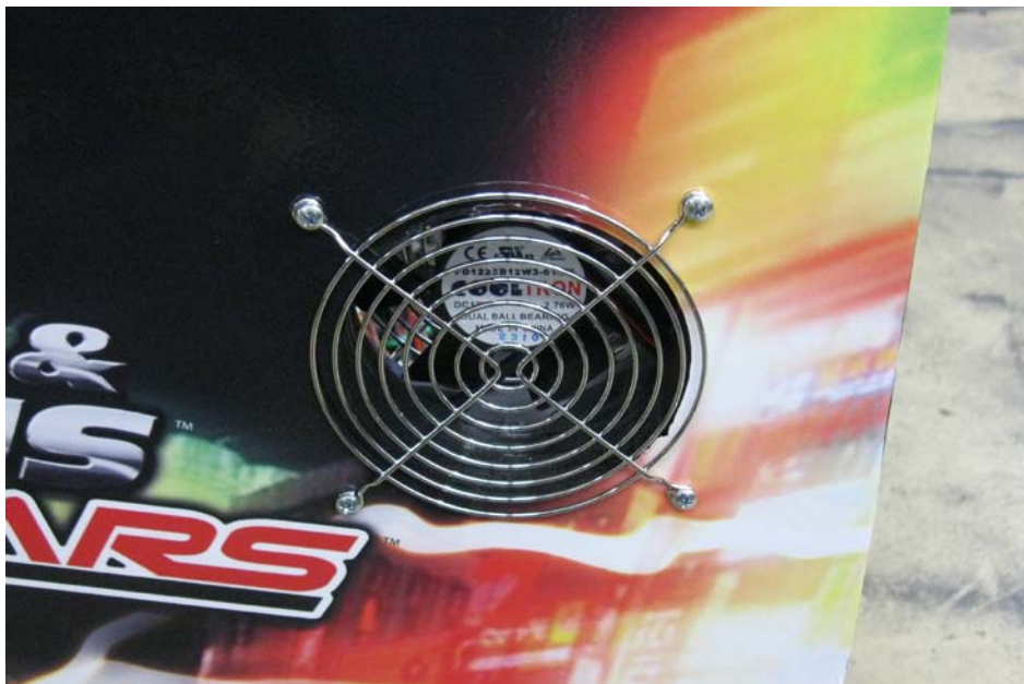
Figure 35 - DO NOT INSTALL FAN GUARD ON OUTSIDE AS SHOWN
