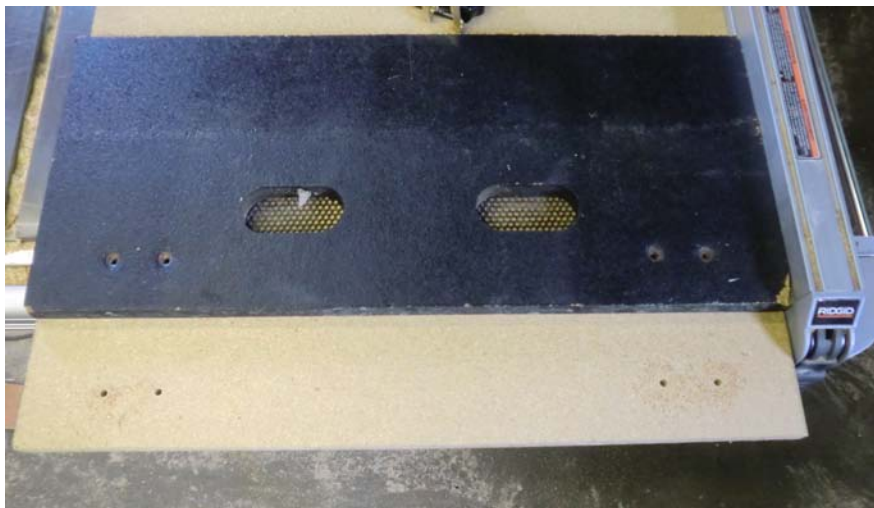
Figure 75 - Drill Holes for Tongue Plates
