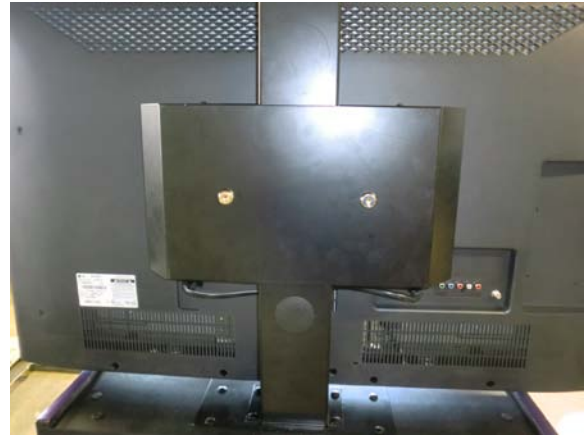
Figure 72 - Install Security Box and Tower Plug
