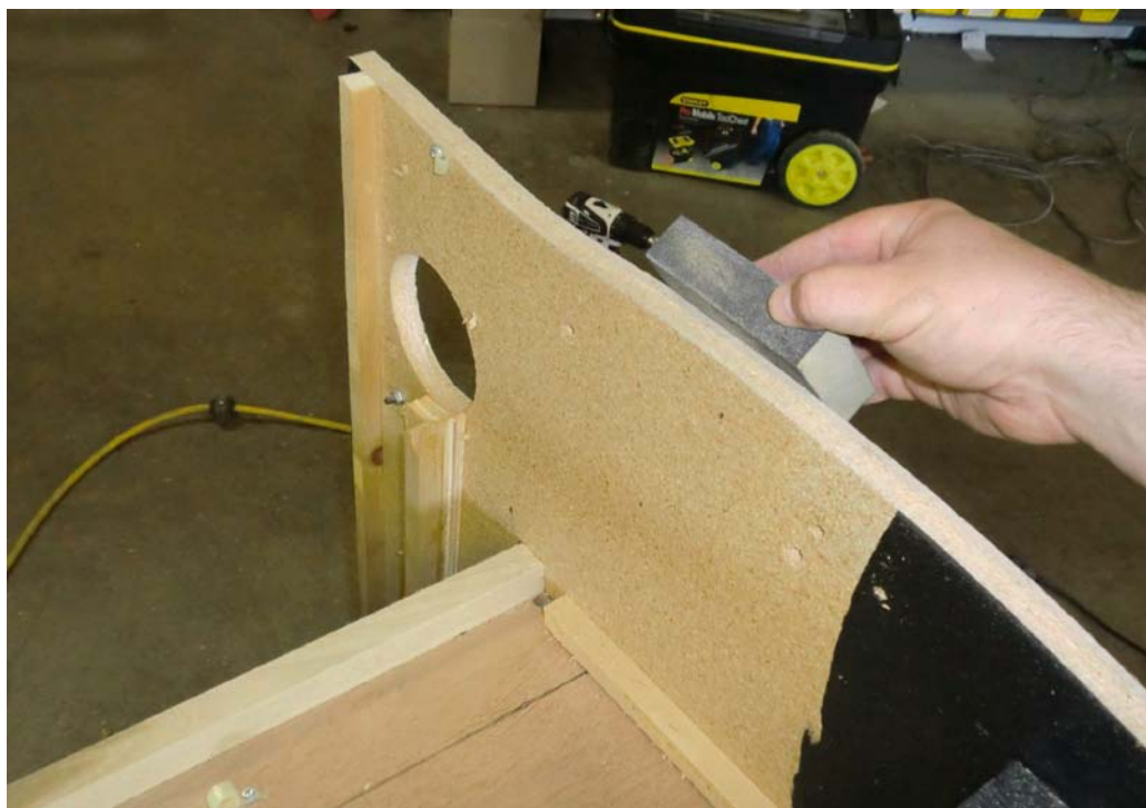
Figure 18 - Sand Cut Edges
