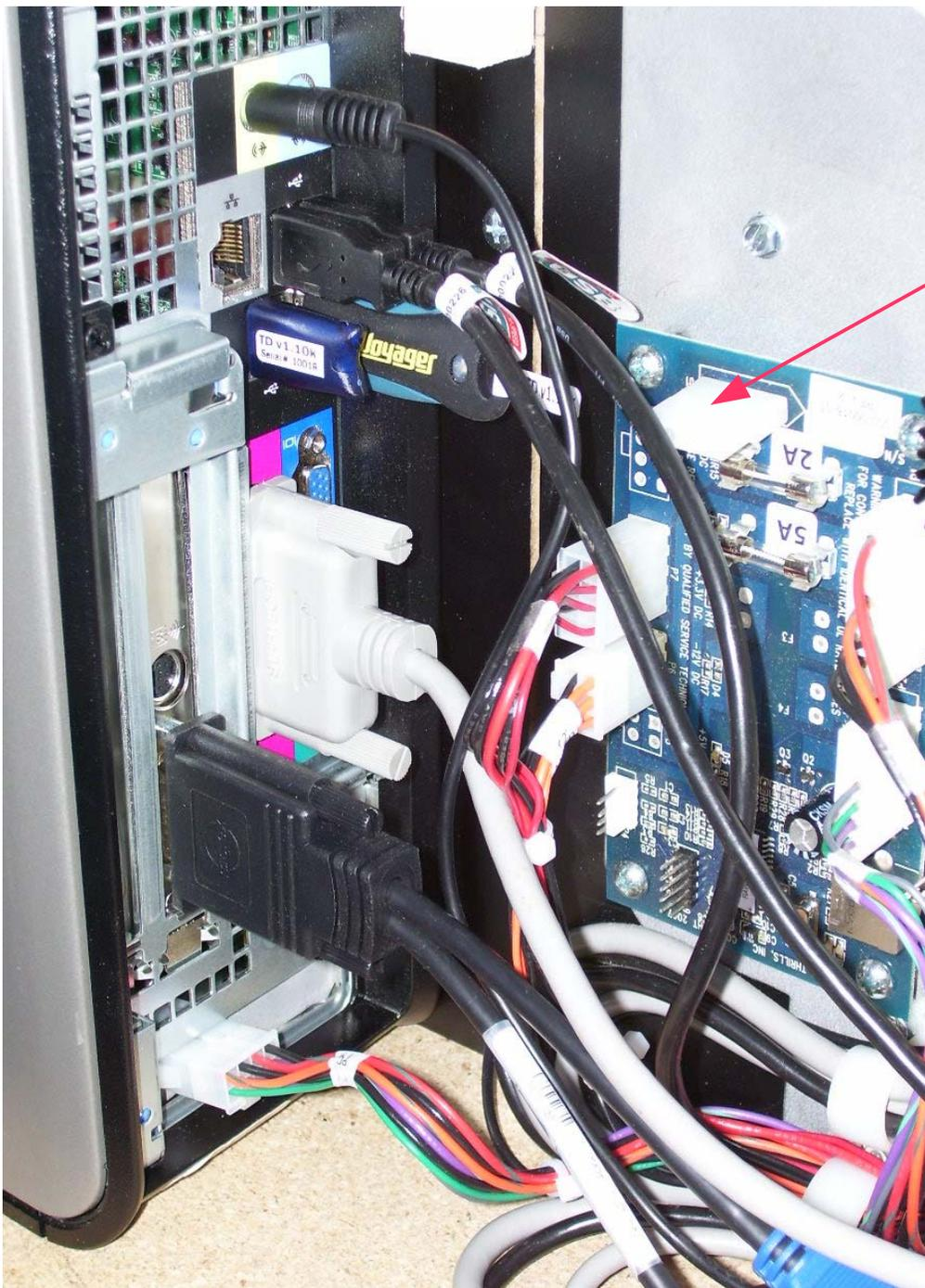
THE CONNECTOR FOR THE FAN PLUGS INTO THE 5-PIN CONNECTOR THAT IS PRESENT ON THE FUSE BOARD. VERIFY THAT IT IS CONNECTED.
