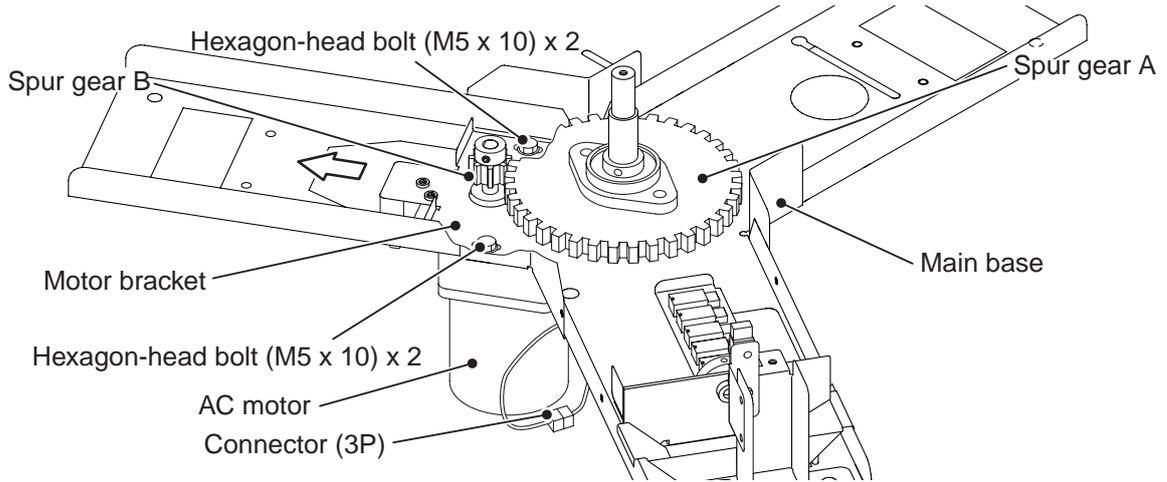
Then, disconnect the connector (3P), remove the two previously loosened hexagon-head bolts (M5 x 10), and remove the motor bracket with the motor from the main base.
