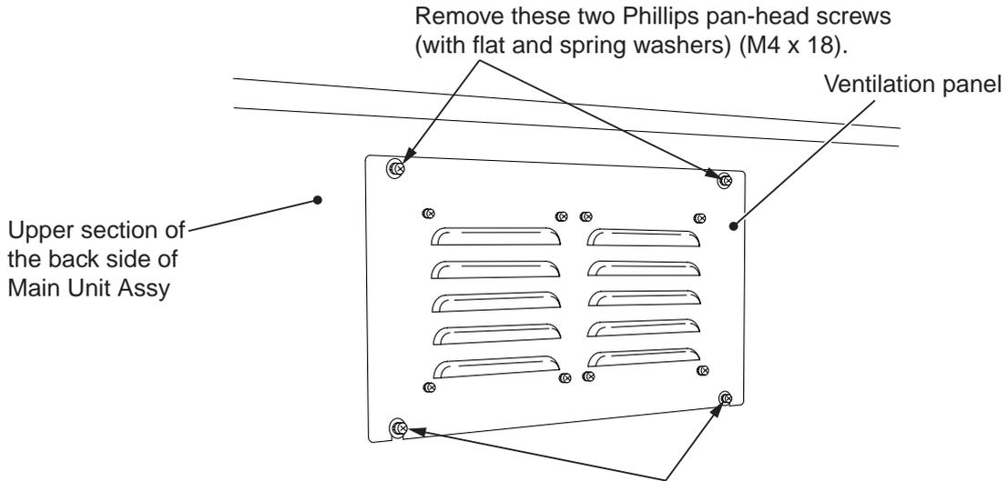
Loosen (do not remove) these two Phillips pan-head screws (with flat and spring washers) (M4 x 18).
