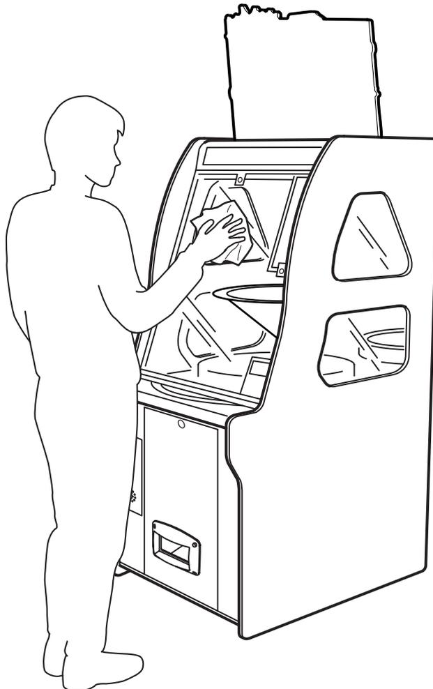
**8-1-3 Cleaning the coin selector - To be conducted by a technician only -****! WARNING**
