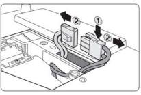
6. Lift the handle so that it stands up. Use the handle to slowly pull the lamp out of the projector.
