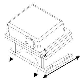
The projector base is mounted with slots so the entire unit can move forward or backward on the **Projector Mount Board**. There is also enough room to aim the projector right or left.
