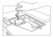
5. Pull out the lamp connector from a slot in the lamp compartment. Disconnect it from the projector as illustrated.
