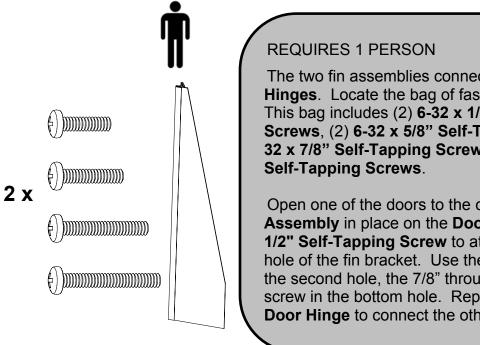
The two fin assemblies connect to the two Door Hinges. Locate the bag of fasteners labeled Fins. This bag includes (2) 6-32 x 1/2" Self-Tapping Screws, (2) 6-32 x 5/8" Self-Tapping Screws, (2) 6-32 x 7/8" Self-Tapping Screws, and (2) 6-32 x 1"
