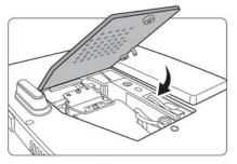
12. Tighten the screws that secure the lamp cover.
