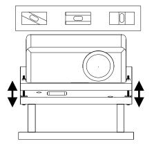
The three bolts circled here are used to change the pitch and to level the projector.
