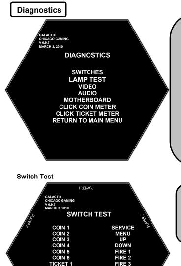
**Switches** – Select this option to test the functionality of the switches.
