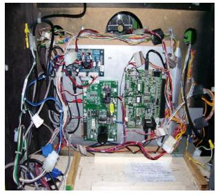
2. LOCATE THE KIT ELECTRONICS PLATE ASSY. REMOVE AND REPLACE THE JAMMA HARNESS WITH THE ONE PROVIDED WITH THE ADDER KIT. INSERT PRE-TERMINATED JAMMA PINS (AUDIO OUTPUT)INTO JAMMA EDGE CONNECTOR AS LABELED.
