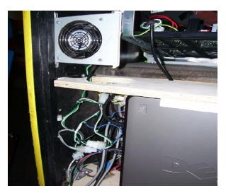
6. USE THE AC Y-CABLE ADAPTOR HARNESS TO CONNECT AC CONNECTION TO PC, MON, COOLING FAN. USE AC ADAPTOR 810-00100-01 AS NEEDED FOR CERTAIN POWER SUPPLIES.
