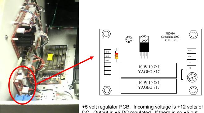
DC. Output is +5 DC regulated. If there is no +5 out check for +12 DC in or +12 out from PE2010X. If +12 is also missing, check 110v in to PE2010X power supply.
