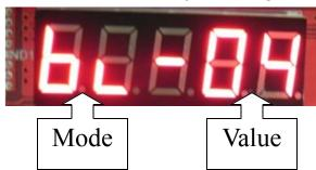
\*\* To save the changes you made to your options you must press the "CLR" button at the screen that showed the version number which is mode UE or mode 1 to exit and save\*\* Pressing the MODE button will erase your changes.
