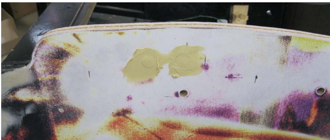
Figure 27 - Fill Preexisting Holes with Wood Filler or Bondo
