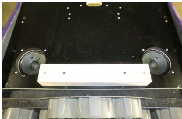
Figure 62 - Install Hood Mounting Block
