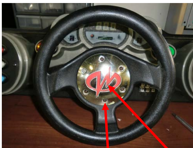
Figure 36 - Remove 6 Screws and Wheel Cap
