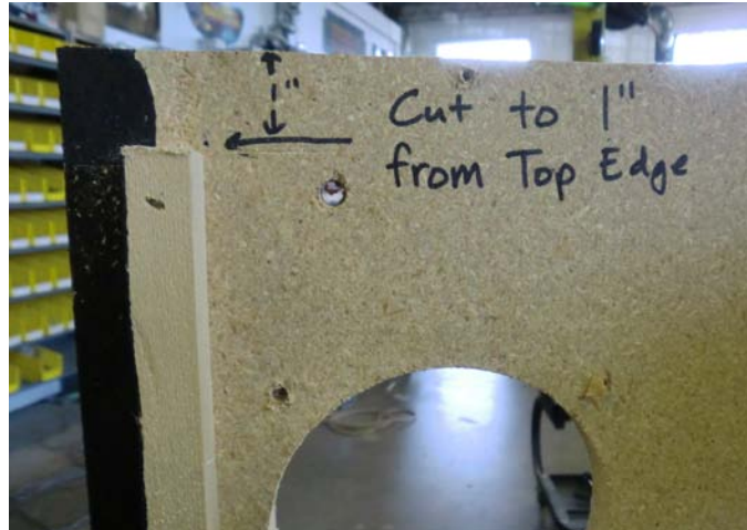
Figure 21 - Cut Rear Door Cleats
