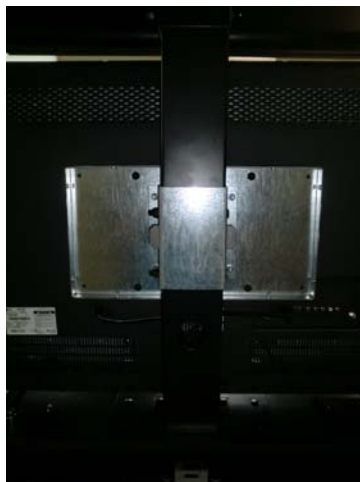
Figure 68 - Monitor Mounted on Narrow Hole Pattern
