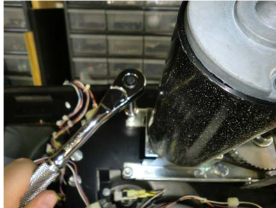
Figure 38 - Remove 4 Flange Nuts to Remove Steering Mech
