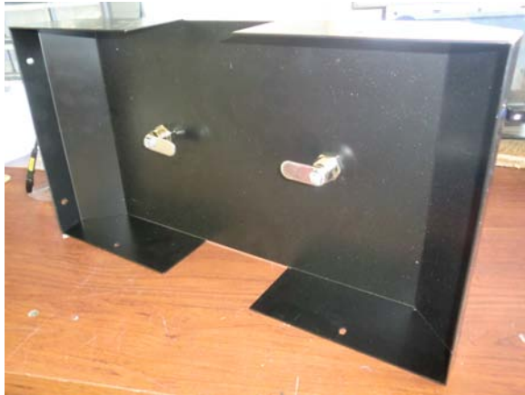
Figure 71 - Install Standard Locks on Security Box
