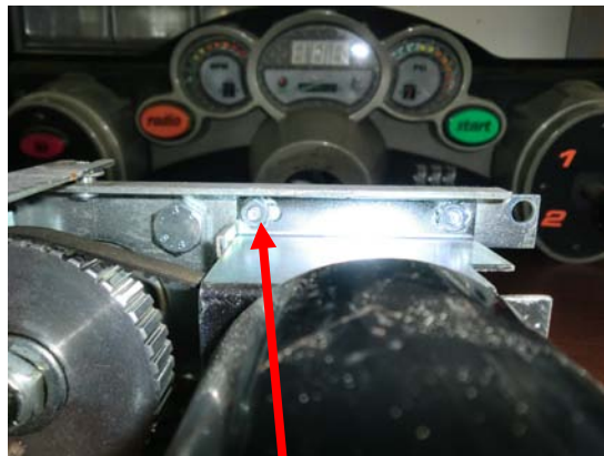
Figure 39 - Loosen 4 Nuts to Replace Timing Belt
