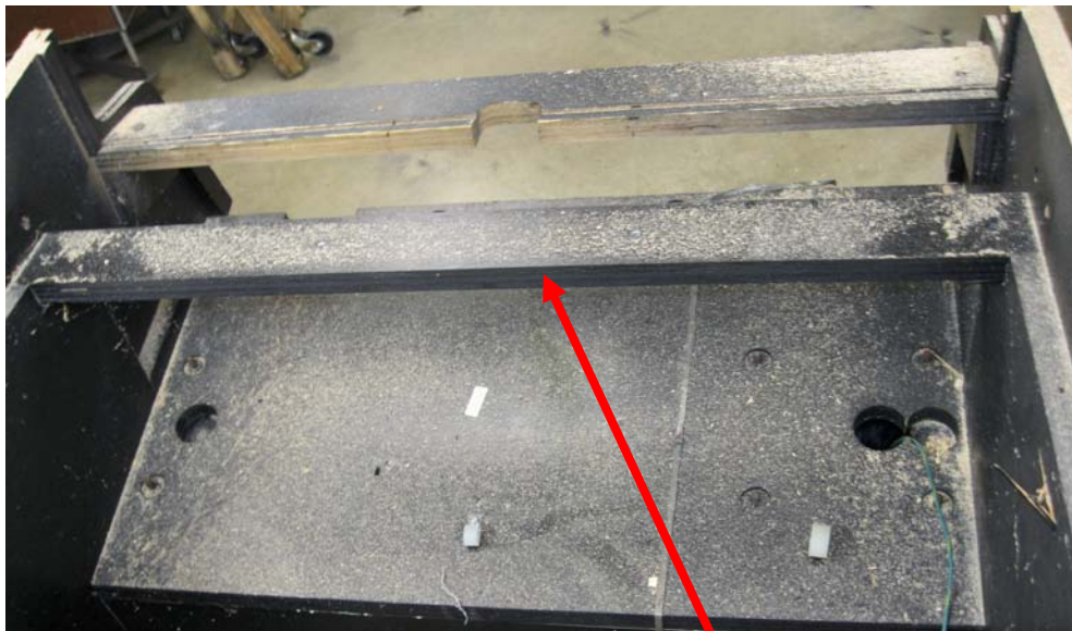
Figure 24 - Remove Support Beam
