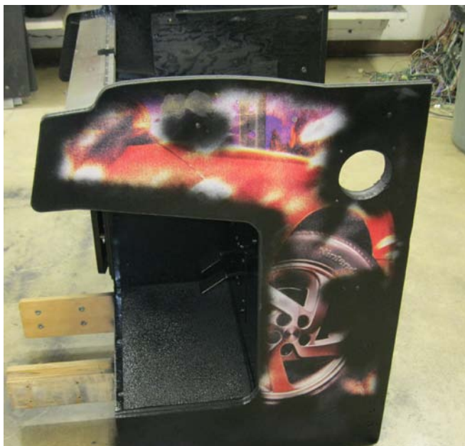
Figure 28 - Paint Edges, Holes, and Sanded Areas
