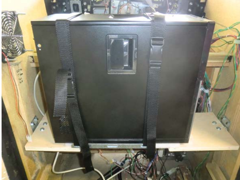
Figure 53 - Proper Mounting of PC Shelf for World & Exotica Conversions
