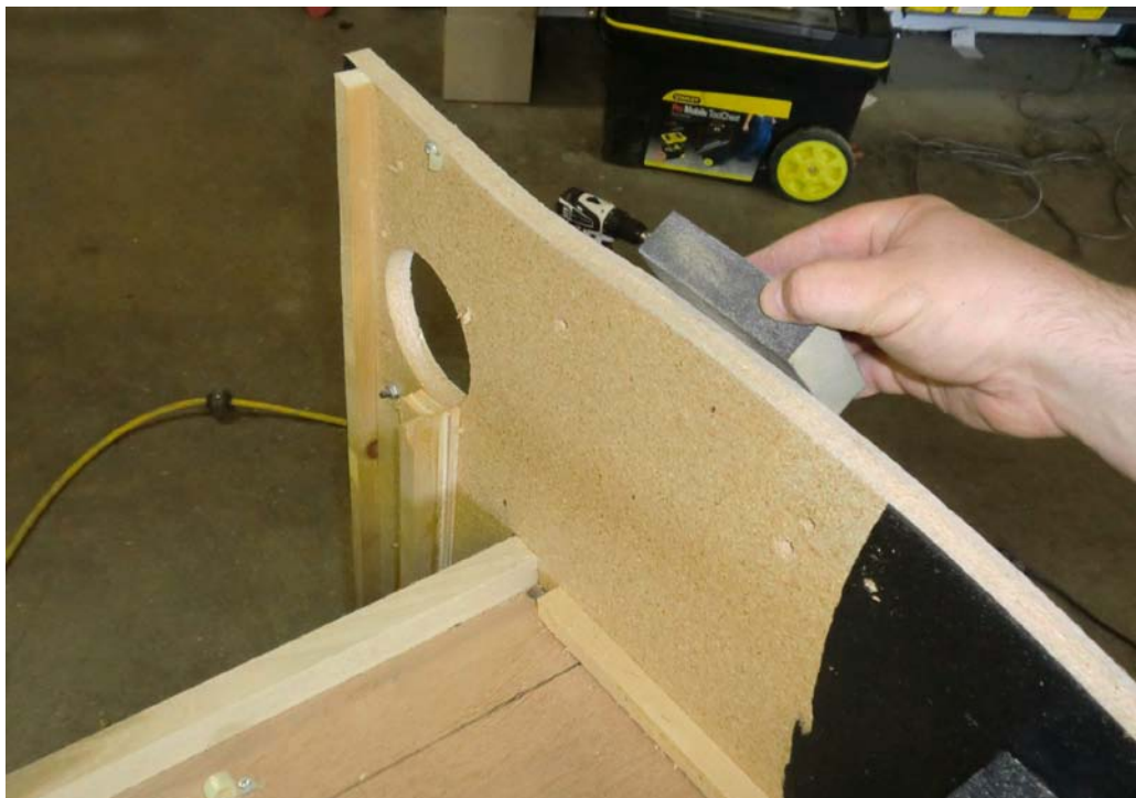
Figure 18 - Sand Cut Edges
