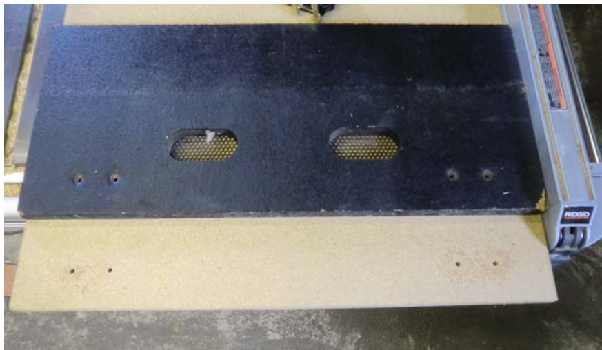
Figure 75 - Drill Holes for Tongue Plates
