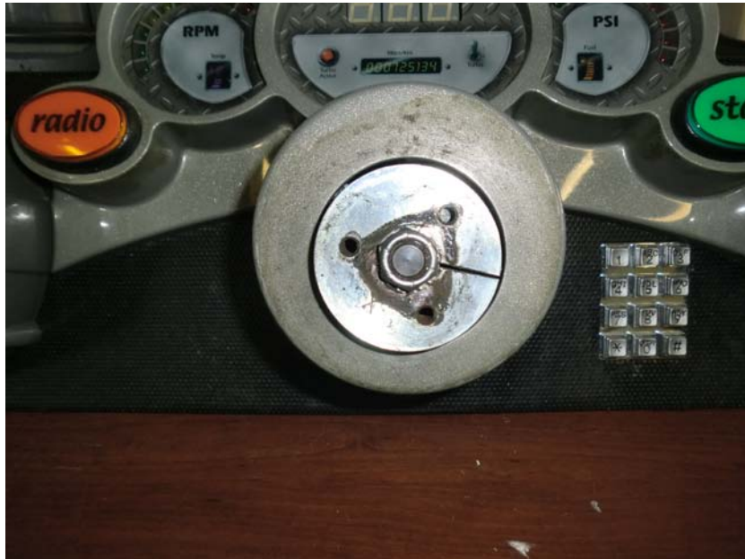
Figure 41 - Tighten Hub Mounting Nut after Steering Mech is Reinstalled
