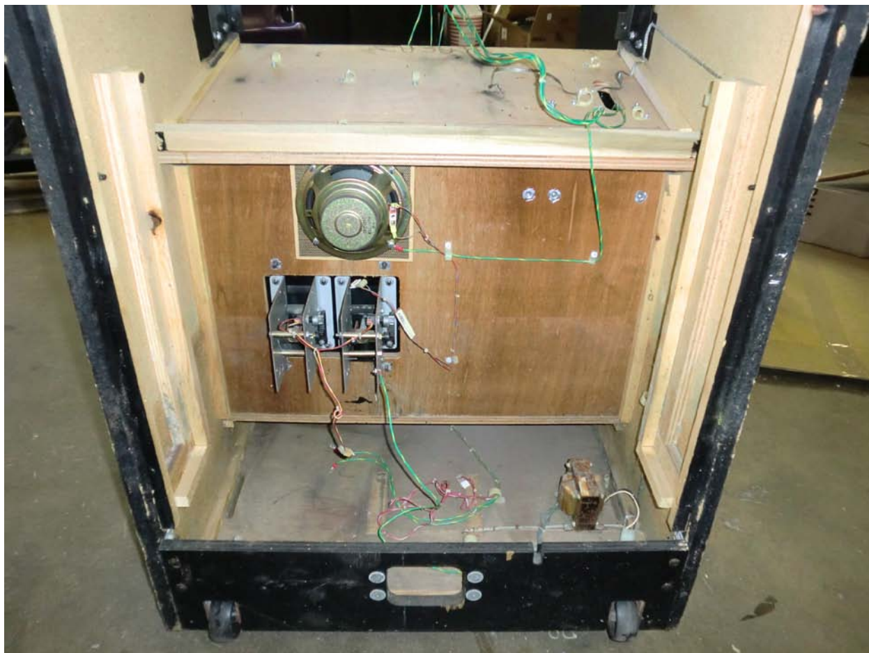
Figure 7 - Remaining Ground Wires
