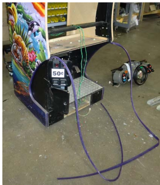
Figure 10 - Pull T-molding Back
