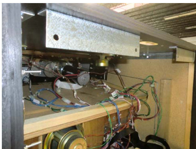
Figure 59 - Install Short L-Brackets
